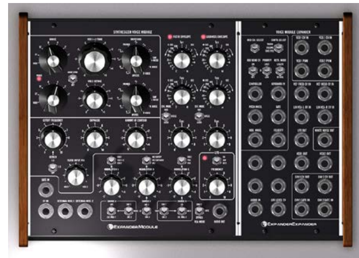
MEM – "Moon Expander Module" in an 8-unit desktop case with "Expander-Expander" for 28 additional insert sockets (rendering).
