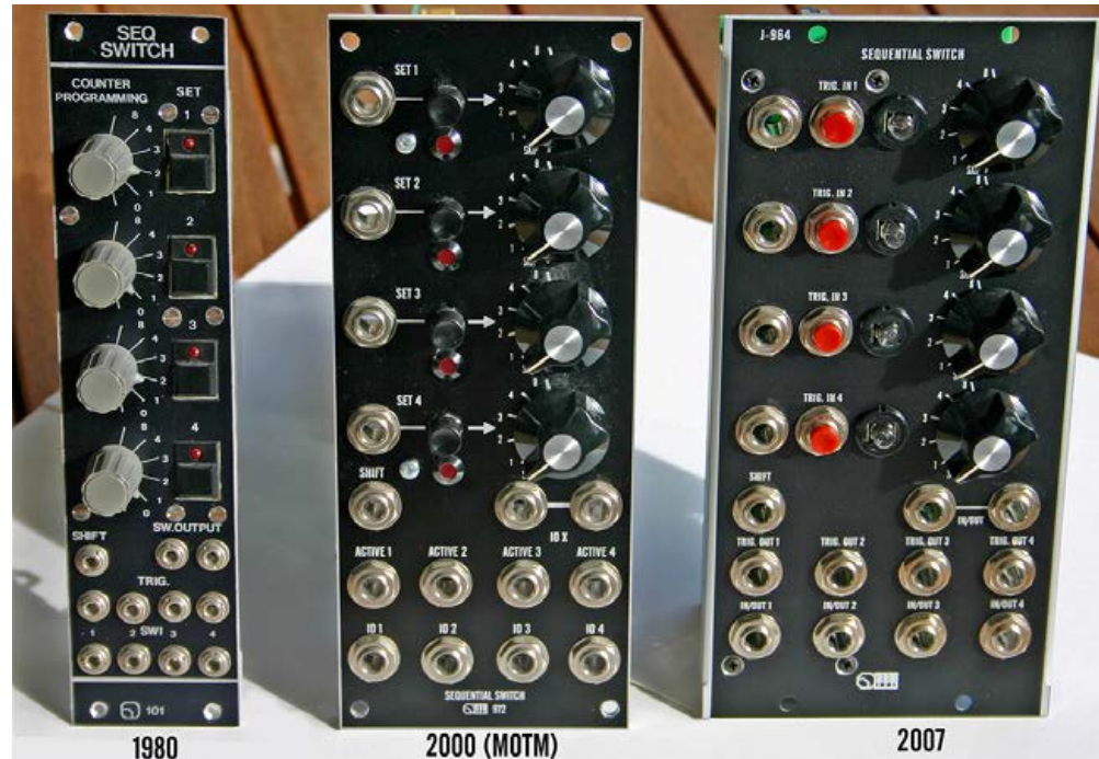
Three incarnations of the Sequential Switch module from 1980, 2000, and 2007. The latter was born in 2008 as Moon M564, the second Moon module.
